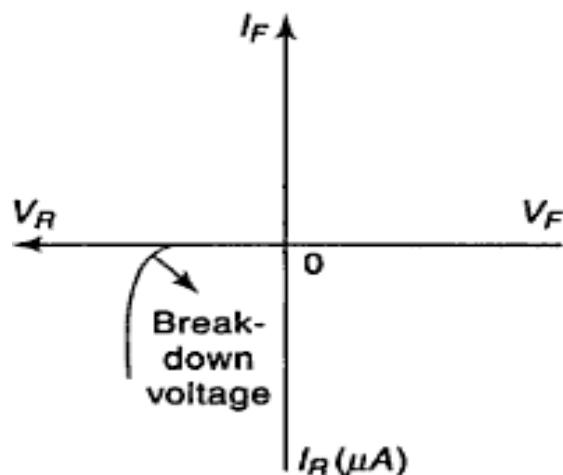
Electrons forming covalent bonds of semiconductor atoms in the P and N type regions may absorb sufficient energy from heat and light to cause breaking covalent bonds. So electron hole pairs continuously produced.
