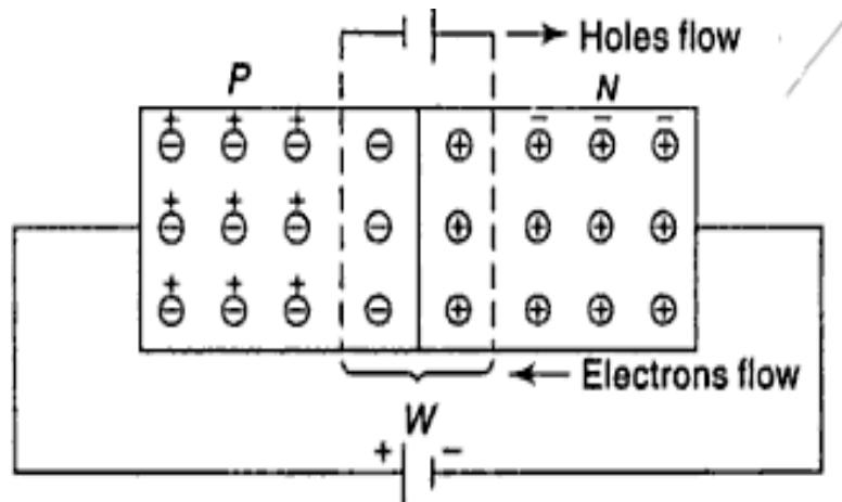
The applied potential in external battery acts in opposition to the internal potential barrier which disturbs the equilibrium.
