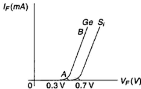
For  $V_F > V_0$ , the potential barrier at the junction completely disappears and hence, the holes cross the junction from P to N type and electrons cross the junction to opposite direction, resulting large current flow in external circuit.
