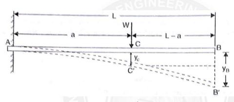
Let  $\theta_C$ = Slope at point C i.e.,  $\frac{dy}{dx}$  at C  $y_C$ = Deflection at point C  $y_B$ = Deflection at point B
