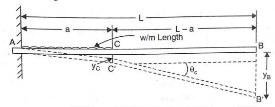
The beam will bend only between A and C, but from C to B it will remain straight since B.M. between C and B is zero. The deflected shape of the cantilever is shown by AC'B' in which portion C'B' is straight.
