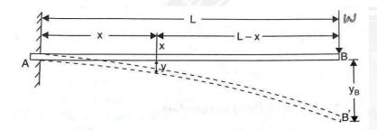
Consider a section X, at a distance x from the fixed end A. The B.M. at this section is given by,
