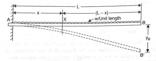
Consider a section X, at a distance x from the fixed end A. The B.M. at this section is given by,
