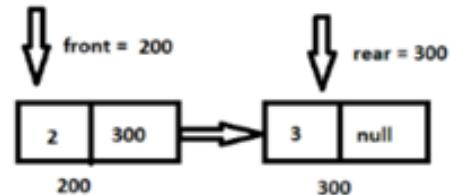
Dequeue an element from the front. Front now points to element with data 2 and rear still points to the last element of the queue.
