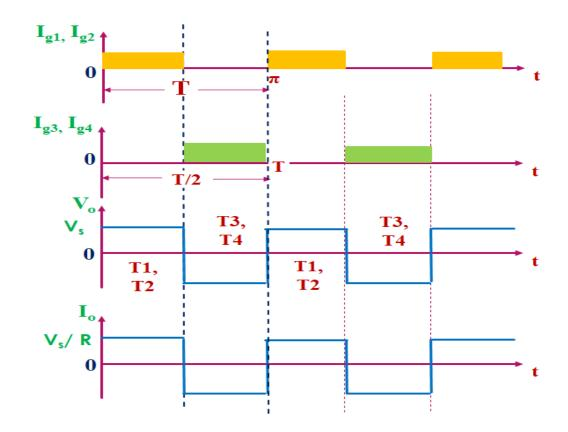
The working operation of Full bridge for pure resistive load is simplest as compared to all loads. As there is not any storage component in the load so, only control switches operate while feedback diodes do not operate through the operation of the inverter. Only two modes are enough for understanding the working operation of a full bridge inverter for R load.
