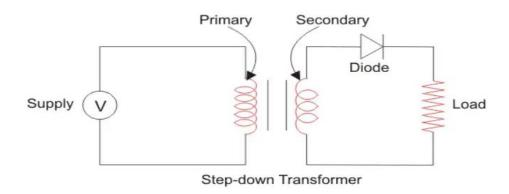
During the positive half-cycle of the AC voltage, the diode becomes forward biased, allowing current to flow through. Conversely, in the negative half-cycle, it is reverse biased, which blocks the current. The resulting DC output waveform from this process is displayed
