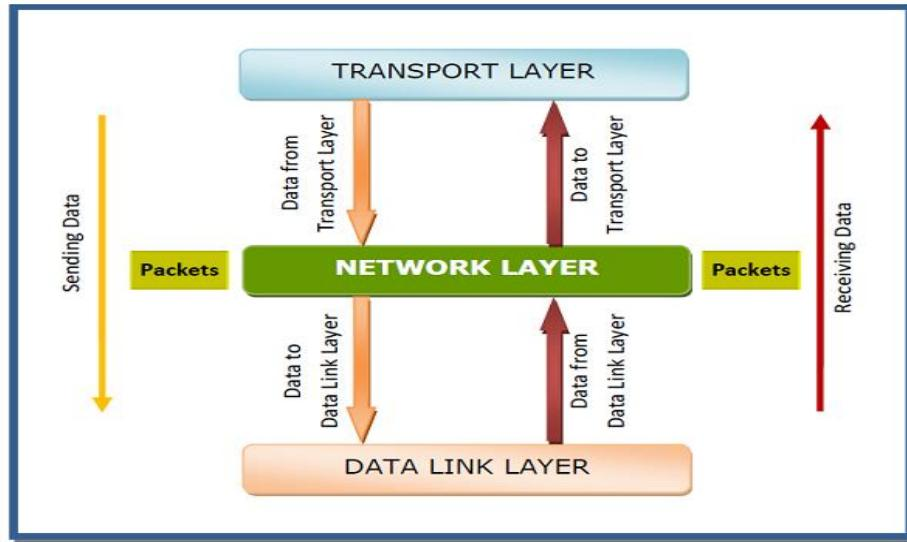
The network layer (Layer 3 of the OSI model) is responsible for end-to-end communication across different networks, a task accomplished through three primary, interconnected functions: **logical addressing, routing, and forwarding**.
