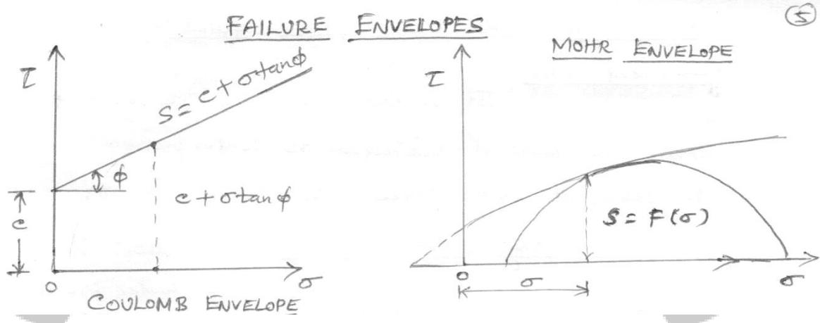
**Coulomb** considered, that the relationship between shear strength and **normal** stress, is represented by a **straight line**.
