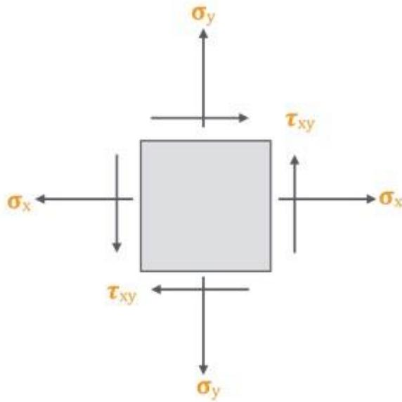
Using a graphical approach, we are able to determine the PRINCIPAL STRESSES on each plane using a MOHR'S CIRCLE.
