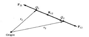
Fig 18: Coulomb vector force on point charges Q1 and Q2
