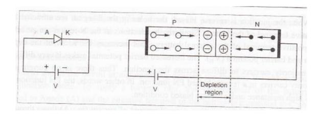
When the junction is forward biased, the holes in the p-region are repelled by the positive terminal of the battery and are forced to move towards the junction. similarly, the electrons in the N-region are repelled by the negative terminal of the battery and are forced to move towards the-junction. This reduces the width of the depletion layer and barrier potential.
