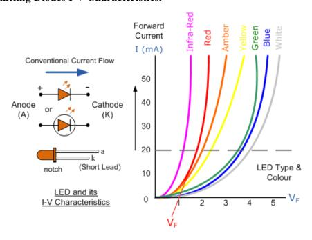
Fig: Light Emitting Diode (LED) Schematic symbol and I-V Characteristics Curves showing the different colours available
