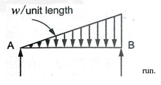
For numerical problem solving, the total UVL is converted into a point load as the area of the triangle and it acting at the C.G of the triangle. Take at a distance of 2/3 of total load acting from zero load.
