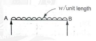
For numerical problem solving, the total UDL is converted into a point load acting at the centre of load.
