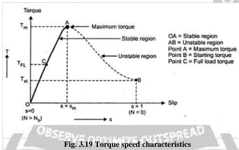
Fig. 3.19 Torque speed characteristics
