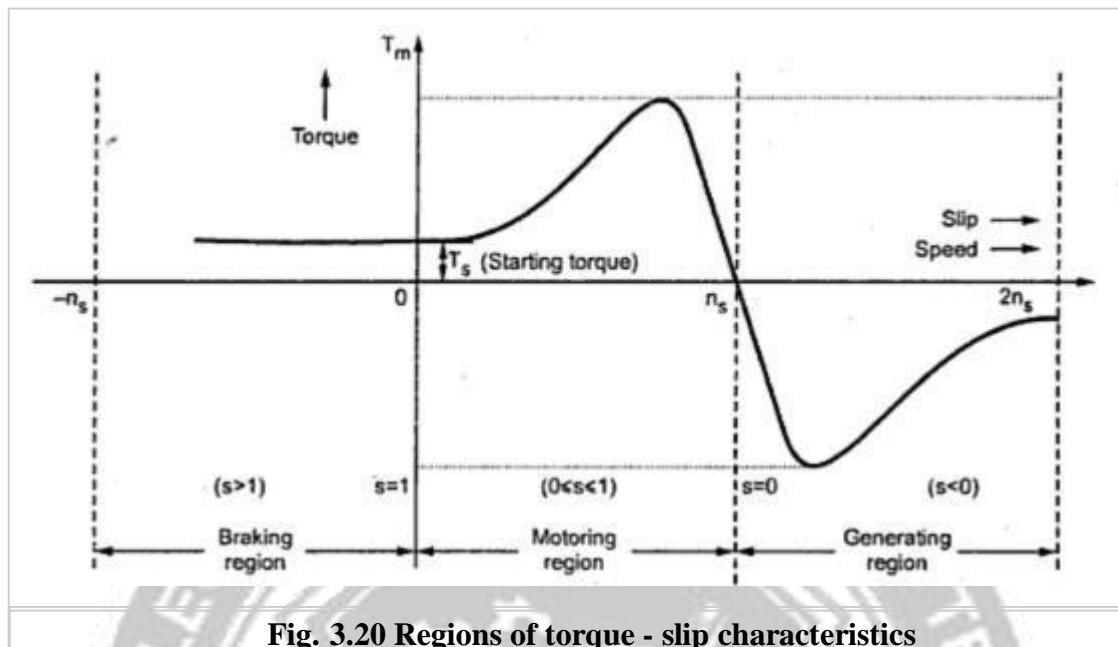
Fig. 3.20 Regions of torque - slip characteristics
