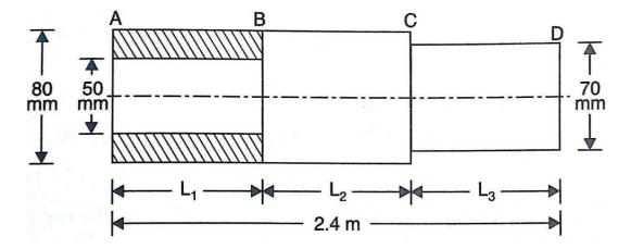
Let Shaft a AB = shaft 1, shaft BC = shaft 2 and shaft CD = shaft 3
