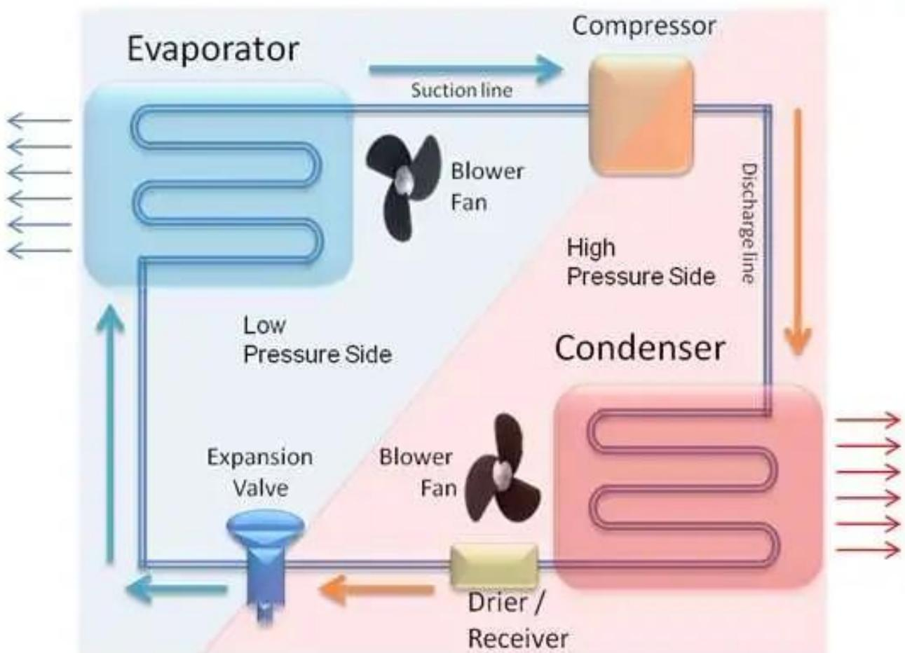
The basic principle behind the operation of HVAC unit is conduction and convection. Heat is transferred from a low-temperature region to a high-temperature region in the car, due to the pressure difference. This process of heat transfer is called Refrigeration. Figure 1 shows the cycle diagram of the complete refrigeration process. An air conditioning system comprises five major components:
