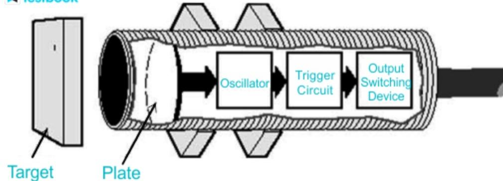
The sensor body, sensing face, indicator light, and cable or cable connection end are the four main components of capacitive proximity sensors.
