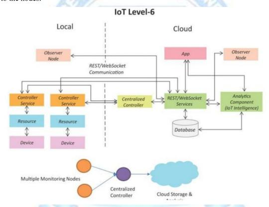
The analytics component analyzes the data and stores the results in the cloud database. The results are visualized with the cloud-based application. The centralized controller is aware of the status of all the end notes and send control commands to the notes.
