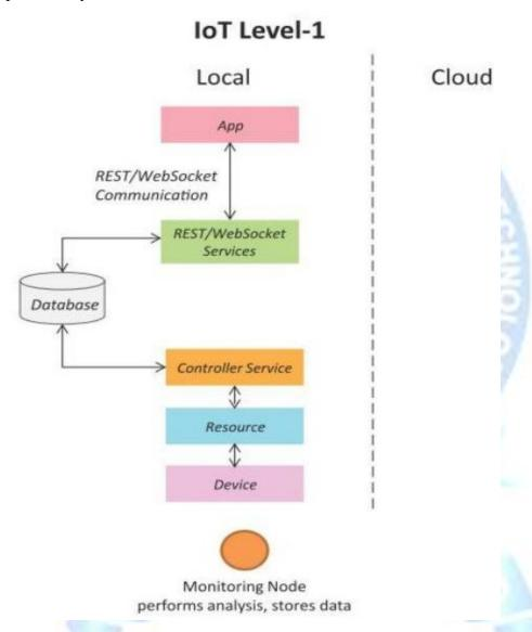
Let us now consider done example of Level 1 IoT **system for home automation**. This system consists of the single node that allows controlling the lights and appliances in your home remotely. The device used in this system interface with their lights and appliances using electronic relay switches.
