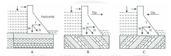
The most unfavourable strike direction is the one in which the beds strike parallel to the axis of the dam and the dip is downstream
