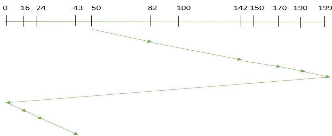
So, the total overhead movement (total distance covered by the disk arm) is calculated as:
