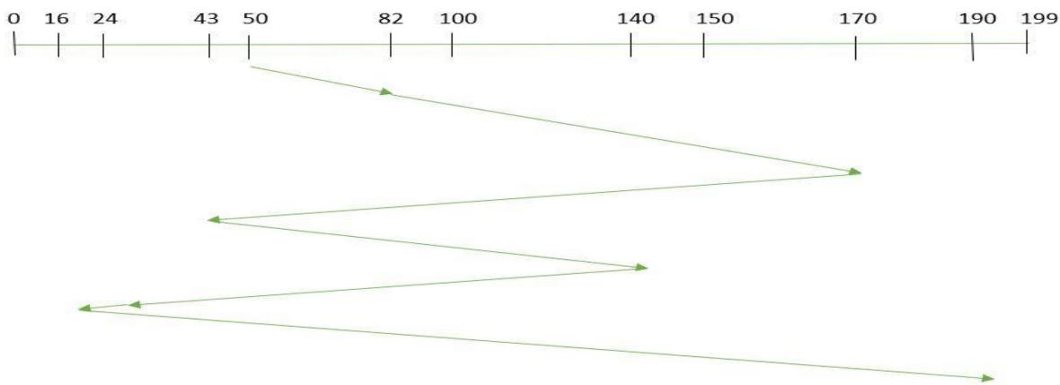
So, total overhead movement (total distance covered by the disk arm) =  $(82-50)+(170-82)+(170-43)+(140-43)+(140-24)+(24-16)+(190-16) = 642$
