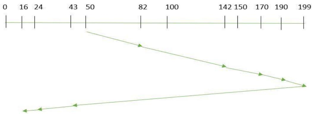
Suppose the requests to be addressed are-82,170,43,140,24,16,190. And the Read/Write arm is at 50, and it is also given that the disk arm should move "**towards the larger value**".
