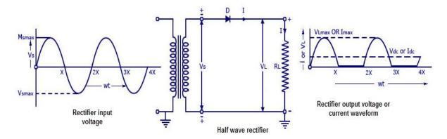
For a sinusoidal input voltage, the no-load output DC voltage for an ideal half-wave rectifier **is**
