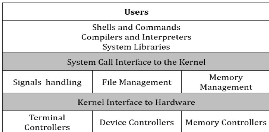
**Fig: Unix - Monolithic Structure**
