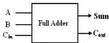
Block schematic of full-adder
