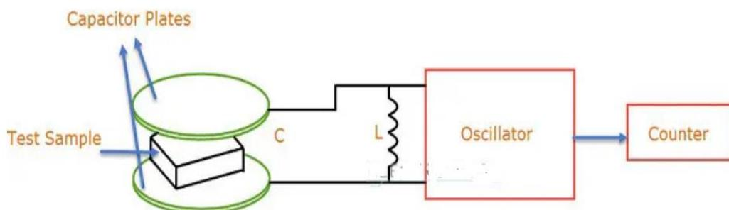
The space between the capacitor plates is usually filled with an appropriate dielectric material (isolator), whose dielectric constant varies when it is subjected to change in humidity.
