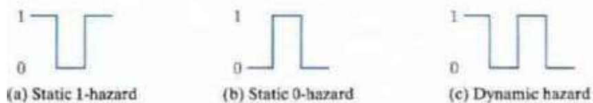
Fig 4.29 – Static and Dynamic Hazard
