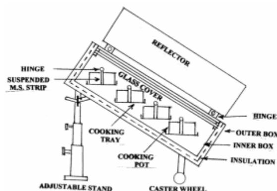
Fig-: Schematic Representation of Solar Cooker
