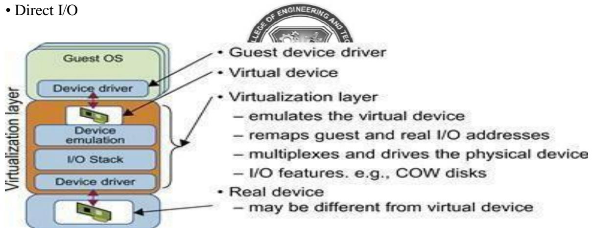
Device emulation for I/O virtualization implemented inside the middle layer that map real I/O devices into the virtual devices for the guest device driver to use.
