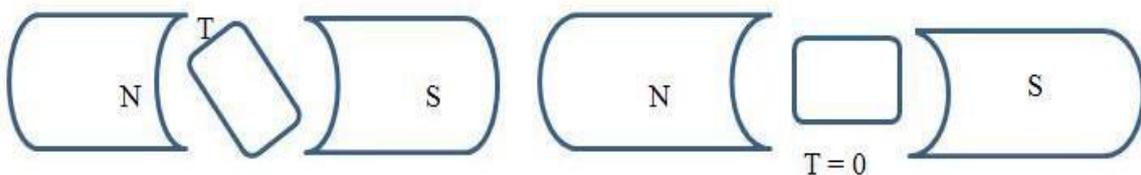
**Figure 5.1.7 Rotor position due to revolving magnetic field**
