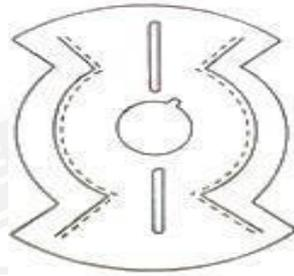
**Figure 5.1.5 cross section of Radially laminated Rotor**
