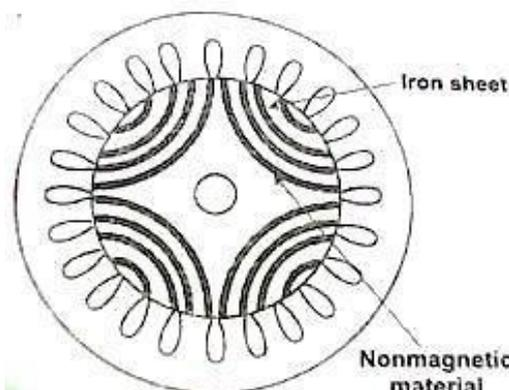
**Figure 5.1.2 cross section of synchronous reluctance motor**
