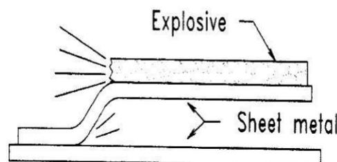
**Figure 5.1.7 Explosion bonding**
