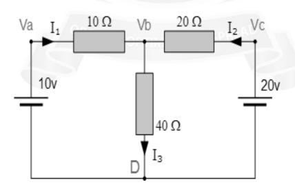
In the above circuit, node D is chosen as the reference node and the other three nodes are assumed to have voltages, Va, Vb and Vc with respect to node D. For example;
