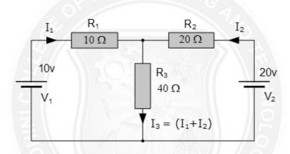
One simple method of reducing the amount of math's involved is to analyse the circuit using Kirchhoff's Current Law equations to determine the currents,  $I_1$  and  $I_2$  flowing in the two resistors. Then there is no need to calculate the current  $I_3$  as its just the sum of  $I_1$  and  $I_2$ . So Kirchhoff's second voltage law simply becomes:
