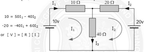
These equations can be solved quite quickly by using a single mesh impedance matrix Z. Each element ON the principal diagonal will be "positive" and is the total impedance of each mesh. Where as, each element OFF the principal diagonal will either be "zero" or "negative" and represents the circuit element connecting all the appropriate meshes.
