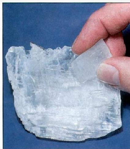
The harder white mineral (calcite) scratches the softer one (gypsum). (Adapted from Jones, 2001: Laboratory Manual for Physical Geology, 3rd edition.)
