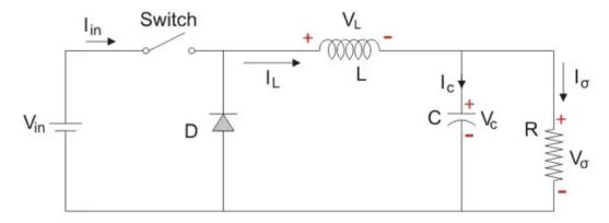
Let us now analyse the **Buck converter** in steady state operation for Mode II using KVL.
