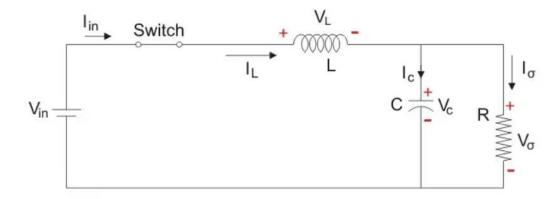
The voltage across the capacitance in steady state is equal to the output voltage. Let us say the switch is on for a time  $T_{\rm ON}$  and is off for a time  $T_{\rm OFF}$ . We define the time period,  $T_{\rm oFF}$ , as  $T = T_{\rm ON} + T_{\rm OFF}$  and the switching frequency,
