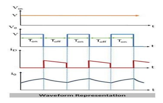
The **Buck converter** has two modes of operation. The first mode is when the switch is on and conducting.
