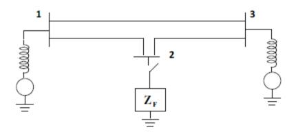
When the fault is simulated, there will be currents in different elements and the bus voltages will be different from 1.0 p.u. These changes have occurred because of i) Generator voltages and ii) Fault current. Any general power system with a number of generators and N number of buses subjected to symmetrical fault at pth bus will be represented as shown in Fig.
