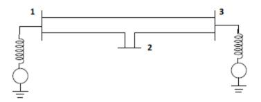
If the generator reactances are included with the transmission network, Zbus matrix of the combined network can be obtained. As stated earlier, there is no current flow in the network in the pre-fault condition and all the bus voltages will be 1.0 p.u. Consider the network shown in Fig. Symmetrical fault occurring at bus 2can be simulated by closing the switch shown in Fig. Here Zf is the fault impedance.
