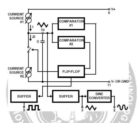
Fig: Functional block diagram of Function generator
