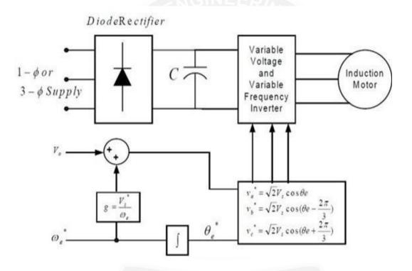
Figure 3.2.1Open loop V/F Control for an IM
