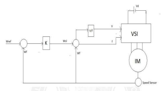
Figure 3.2.2 Closed loop V/F control for an IM (Source: "Fundamentals of Electrical Drives" by G.K.Dubey, page-189)
