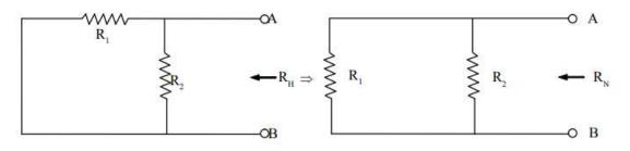
$$\therefore R_{N} = \frac{R_{1}R_{2}}{R_{1} + R_{2}}$$
