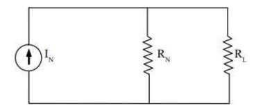
$$I_{L} = I_{N} \frac{R_{N}}{R_{N} + R_{L}} \tag{8}$$
