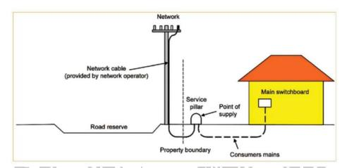
Underground Residential Distribution Systems (URD Systems) refer to electrical power distribution systems designed to deliver electricity to residential areas through underground cables instead of overhead power lines. URD systems have become increasingly popular in urban and suburban areas due to various advantages they offer over traditional overhead distribution systems.
