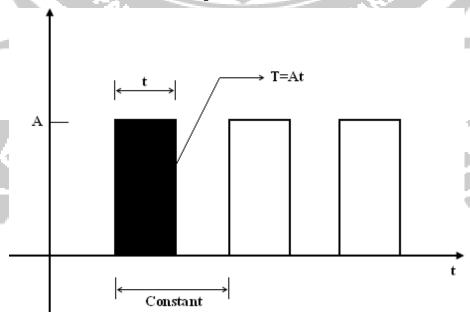
In this method, the pulse width of a pulse train is made proportional to one input voltage and the pulse amplitude is made proportional to the second input voltage. Therefore,  $V_x = K_x A$ ,  $V_y = K_y t$ , and  $V_z = K_z T$  where  $K_x$ ,  $K_y$ ,  $K_z$  are scaling factors. In figure A is the amplitude of the pulse, t is the pulse width and T is the area of the pulse. Therefore,
