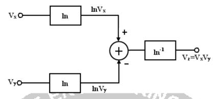
As shown in figure the input voltages  $V_x$  and  $V_y$  are converted to their logarithmic equivalent, which are then added together by a summer. An antilogarithmic converter produces the output voltage of the summer. The output is given by,
