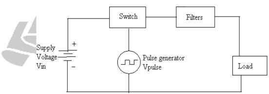
Fig : Basic Switching regulator
