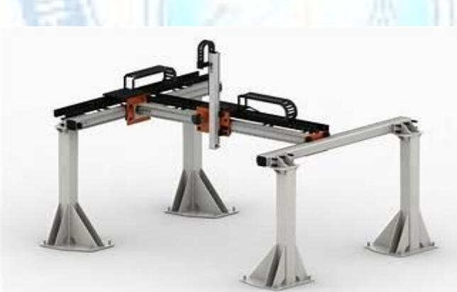
This type of robot is generally mounted direct to the shop floor and usually has a large work envelope. It can be used for material handling applications. They can be pneumatic powered the cost of servo drives for industrial robotics is getting so competitive that today the air powered types are few and far between.
