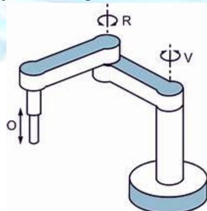
A typical SCARA configuration includes a controller, a power supply, an end-effector (like a gripper or special tool), and specialized software. SCARA robots stand out from other industrial robots due to their unique range of motion, particularly in the X-Y plane. This means it can move horizontally in any direction within its workspace. It can also move vertically, although with some limitations, as the vertical axis remains fixed.
