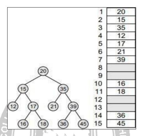
This shows a binary tree and its corresponding sequential representation. The tree has 11 nodes and its height
