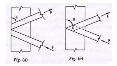
**WELDED CONNECTION Lap Joint** – Overlap should not be less than ¼ times thickness of bar or member, whichever is less. **Butt Joint** – Full penetration butt weld or fillet weld on each side, lacing bar should be placed opposite to flange or stiffening component of main member.
