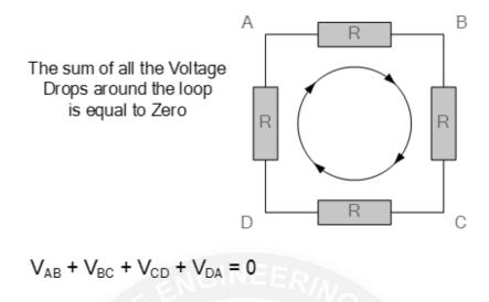
Starting at any point in the loop continue in the same direction noting the direction of all the voltage drops, either positive or negative, and returning back to the same starting point. It is important to maintain the same direction either clockwise or anti-clockwise or the final voltage sum will not be equal to zero. We can use Kirchhoff's voltage law when analysing series circuits.
