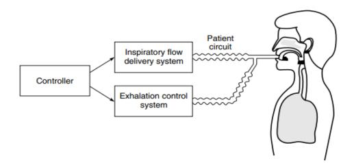
The diagram depicting the components of a ventilator system.
