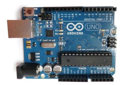
An easy USB interface . The chip on the board plugs straight into your USB port and registers on your computer as a virtual serial port. This allows you to interface with it as through it were a serial device. The benefit of this setup is that serial communication is an extremely easy (and time-tested) protocol, and USB makes connecting it to modern computers really convenient.
