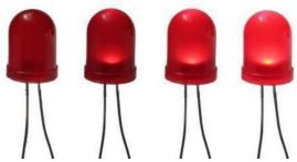
As mentioned earlier, the Arduino has a number of built in special functions. One of thesespecial functions is pulse width modulation, which is the way an Arduino is able to create an analog-like output.
