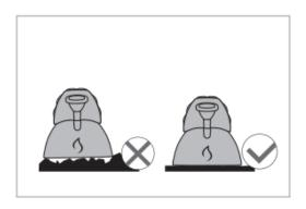
prepare a firm, flat surface clear of obstructions - do not place on soft or unstable ground e.g. flat dry ground, tile, concrete
