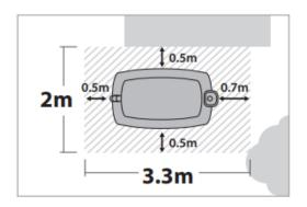
prepare at least 2 x 3.3m space for the system (0.5m side, 0.7m front clearance for maintenance & daily usage)
