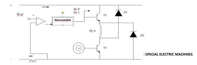
**Figure 2.4.2 (a) voltage PWM type current regulator** [Source: "special electric machines" by R.Srinivasan page:3.53]
