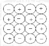
When an electric field is applied, the positive charges are accumulated near the negative electrode as shown in figure.
