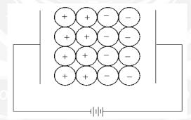
Therefore a dipole moment is induced due to the displacement of the ions. Then the induced dipole moment per unit volume gives the induced polarization. This polarization is known as Space charge polarization
