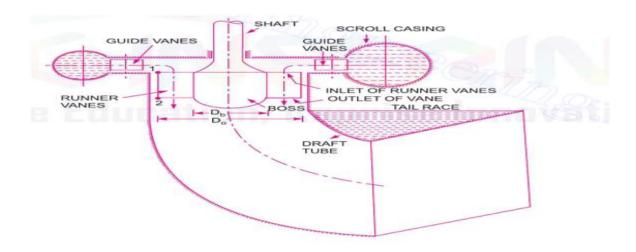
$$Q = \frac{\pi}{4} \left( D_o^2 - D_b^3 \right) \times V_{f_1}$$
