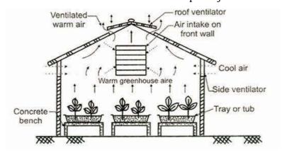
the greenhouse. The ventilators on the roof as well as those on the side wall accounts, each about 10% of the total roof area. During winter cooling phase, the south roof ventilator was opened in stages to meet cooling
