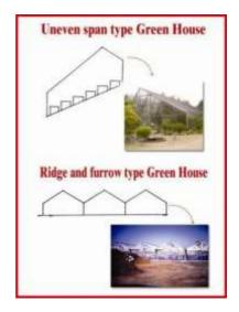
length of the eave (Fig. 2). The eave serves as furrow or gutter to carry rain and melted snow away. The side wall is eliminated between the greenhouses, which results in a structure with a single large interior, Consolidation of interior space reduces labour, lowers the cost of automation, improves personal management and reduces fuel consumption as there is less exposed wall area through which heat escapes. The snow loads must be taken into the frame
