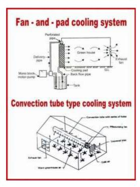
cooling the air everywhere. As this system does not wet the foliage, there is less scope for disease and pest attack. The plants stay dry throughout the process. This system is equally useful for seed germination and propagation since it eliminates the need for a mist system.
