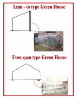
building is extended with appropriate greenhouse covering material and the area is properly enclosed. It is typically facing south side. The lean-to type greenhouse is limited to single or double-row plant benches with a total width of 7 to 12 feet. It can be as long as the building it is attached to. It should face the best direction for adequate sun exposure.
