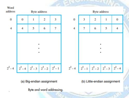
The name big-endian is used when lower byte addresses are used for the more significant bytes (the leftmostbytes) of the word.
