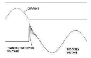
A terminal fault is a fault that occurs at the circuit breaker terminals. The circuit breaker interrupts a short-circuit at current zero, at this instant the supply voltage is maximum and the recovery voltage tends to reach the supply voltage with a high frequency transient. The normalized value of the overshoot or amplitude factor is 1.4.
