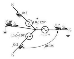
Since the generator is unloaded the internal emfs are Ean = 1.0 $Ebn = 1.0 \angle -1200 Ecn = 1.0 \angle 120^{\circ}$
